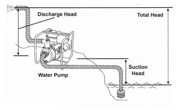
As the head (pumping height) increases, pump output decreases. The length, type, and size of the suction and discharge hoses can also significantly affect Pump output.
